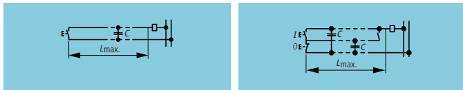
Figure 41: Two-wire control (left) and three-wire (pulsed) control
